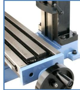
The large mill table provides 50% more table area than other mini mills. It also has 30% more travel in each direction. The resettable feed dials allow you to zero them at any point.
